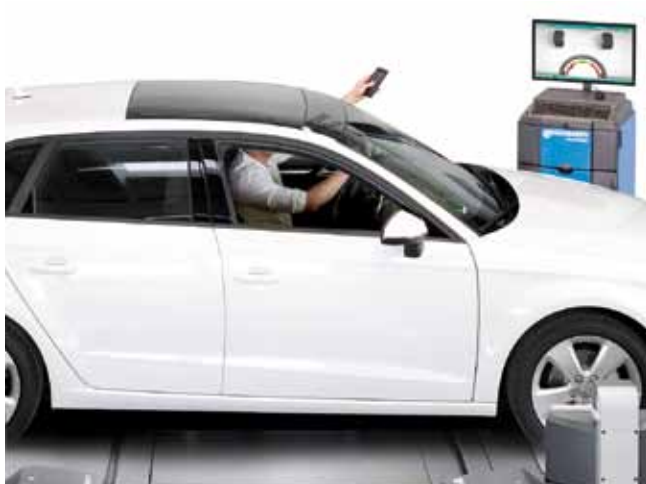
Touchless: wheel alignment from the driver's seat
