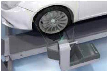
High-frame-rate digital image processing generates a 3D model of the wheel.
